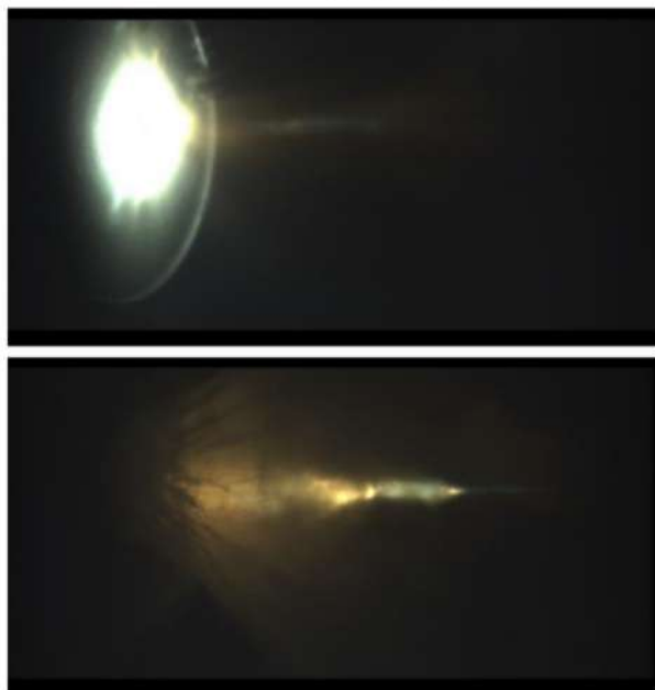
Figure 1: Pictures of a hypervelocity impact flash from a 1 mm stainless steel projectile impacting an ice mixture target at 6.03 \text{ km s}^{-1} . The target mixture consisted of \text{CO}_2 ice, (\text{NH}_4)_2\text{SO}_4 , NaCl and water ice. Top: impact flash, Bottom: subsequent picture frame ( \sim 0.5 \text{ ms} later, post-impact) showing the ejecta and residual light trail.
